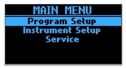
The Main Menu includes three submenus: Program Setup, Instrument Setup and Service:
